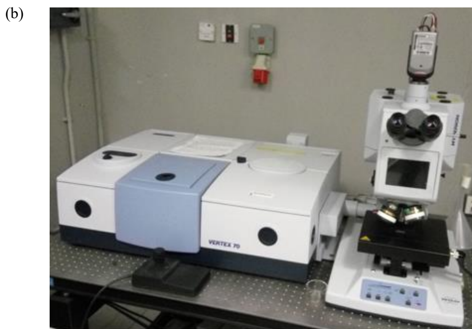
Figure 3.3 Mechanism of the ATR accessory (a) and photography of the Bruker Vertex-70 FTIR (b).
