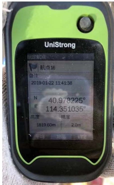
Figure 5.5 Ji Si Bao G128BD Beidou handheld
