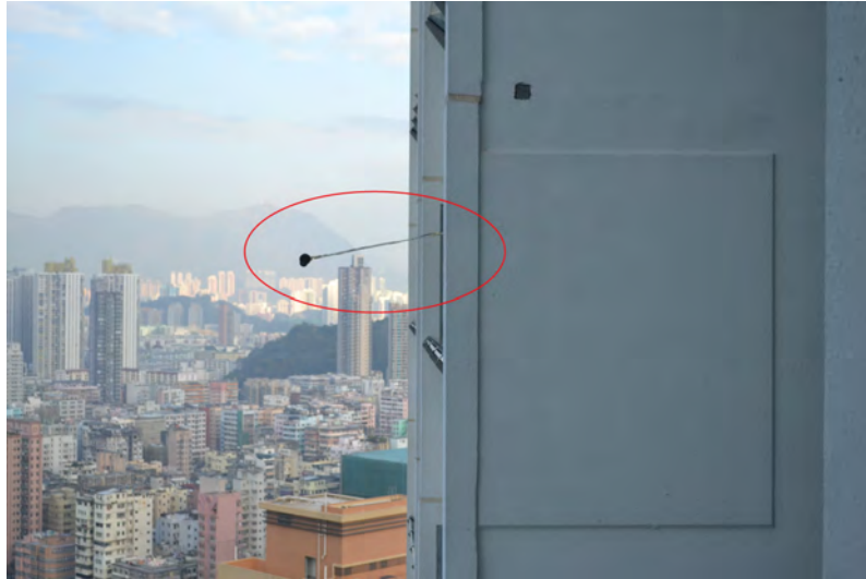
Figure 5.2: The microphone was positioned about one meter outside the building façade. A 1.5-meter stick provided mechanical support to the microphone, with the other end of the stick supported by a tripod. A Bruel and Kjaer windscreen covered the microphone.
