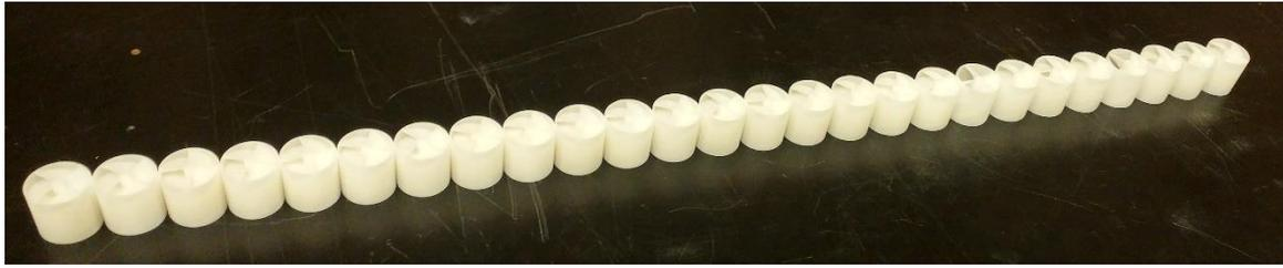
**Fig. 2.19** Gradient helicoid unit cells with a uniform height of 32 mm.
