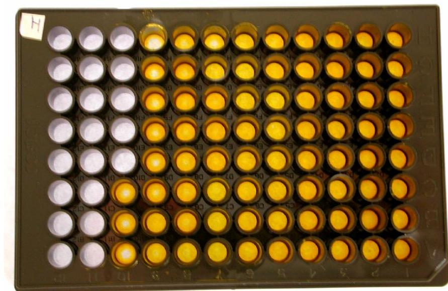
Figure 2.2 A 96-well microtiter plate with some of the microwells coated with ORMOSIL oxygen sensing films.
