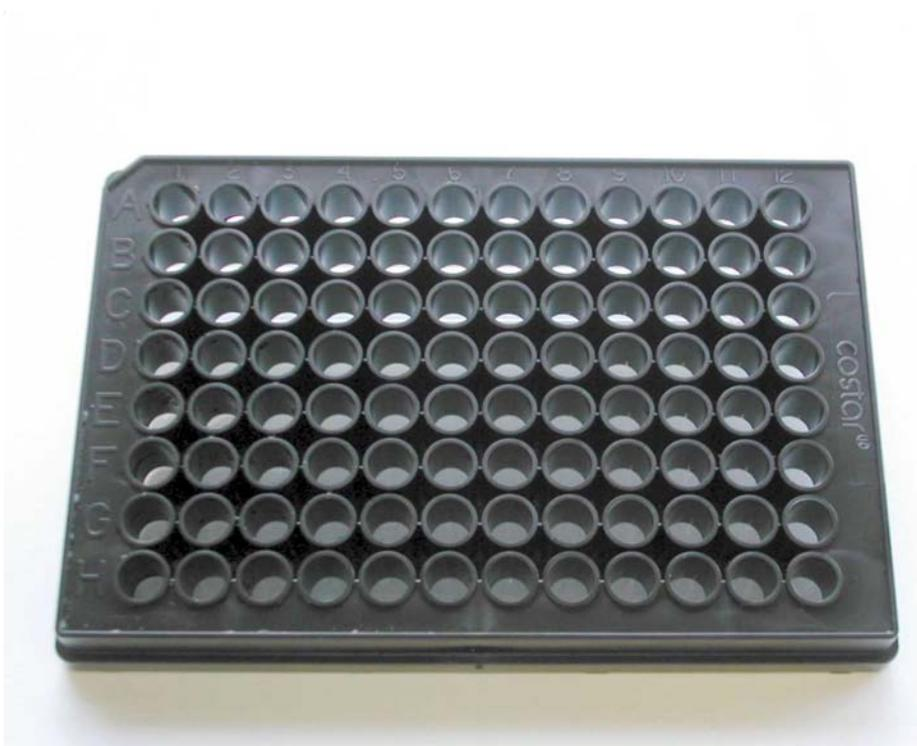
Figure 1.1 A black 96-well microtiter plate with flat clear bottom for fluorescence measurement.
