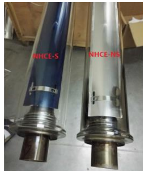
Fig. 2.4 Receiver tubes with different metal radiation shields [121]: with solar selective coating (left) and without solar selective coating (right)
