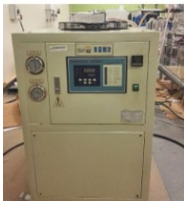
(c) Water chiller
