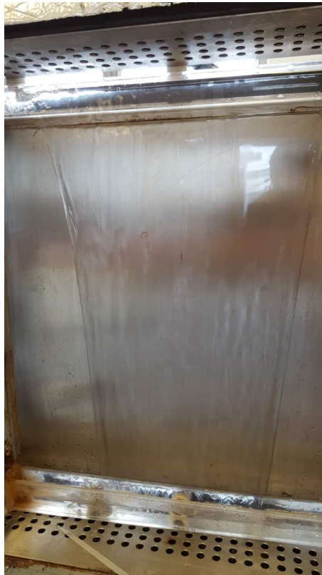
Figure 1.5 Typical falling film
