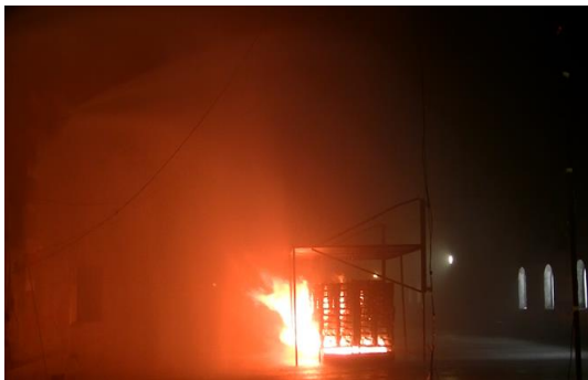
(c) 60 s after activating FFFS
