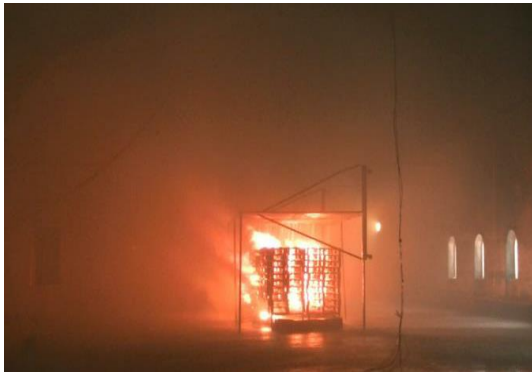
(e) 240 s after activating FFFS
