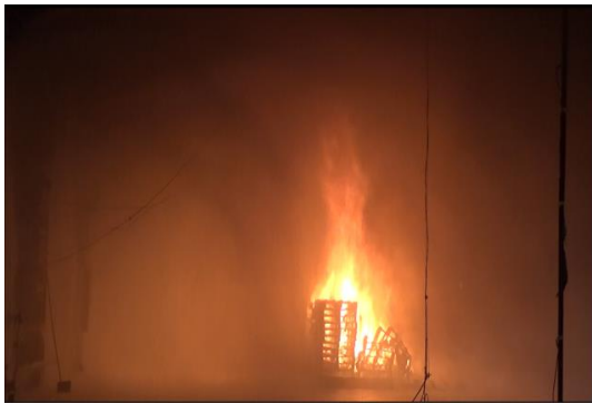
(e) 240 s after activating FFFS
