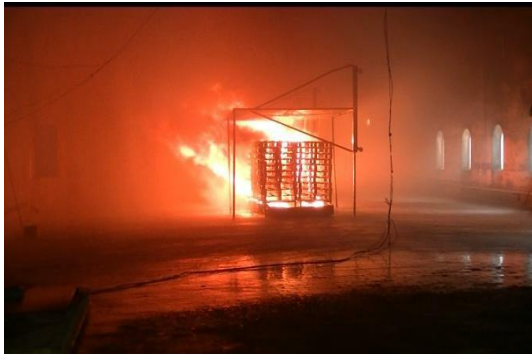
(c) Ventilation system activated at 90s
