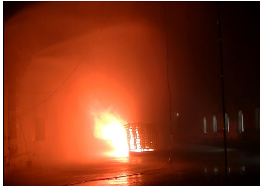
(c) 60 s after activating FFFS
