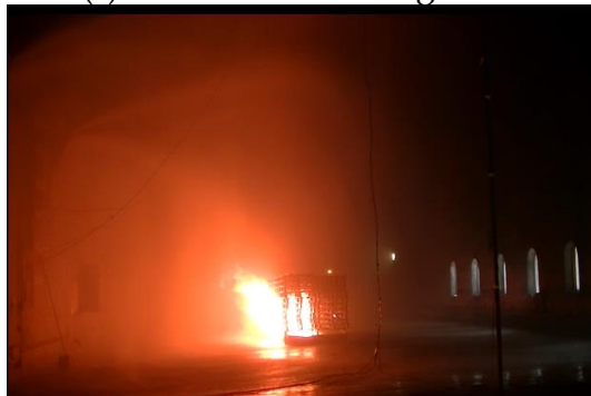
(e) 180 s after activating FFFS
