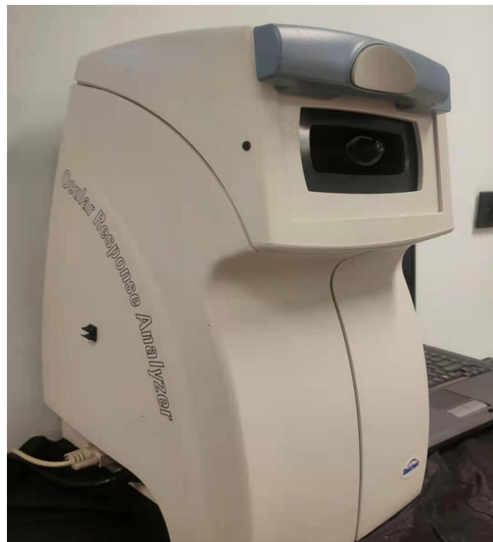
Figure 2.4. The Ocular Response Analyzer (ORA). The ORA contains an infrared light emitter, infrared sensor, air pump, and pressure transducer.
