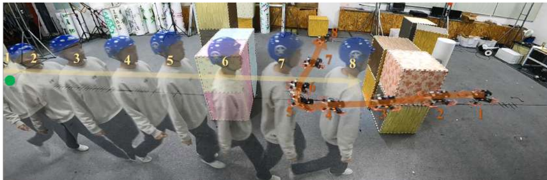
Fig. 5.17.: The composed image of one of the hardware flight tests. The drone takes off from the right side, and the goal is located at the left side, denoted by a green dot. The numbers mark the corresponding frames, increasing with time.
