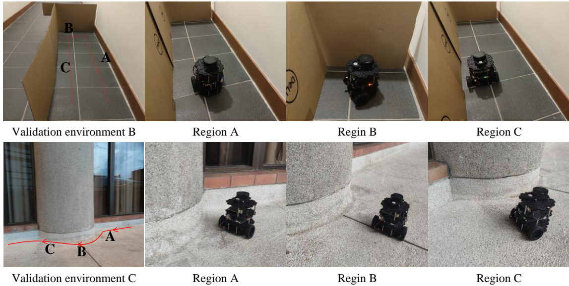
Figure 6. 15 Navigation in narrow regions and curved columns
