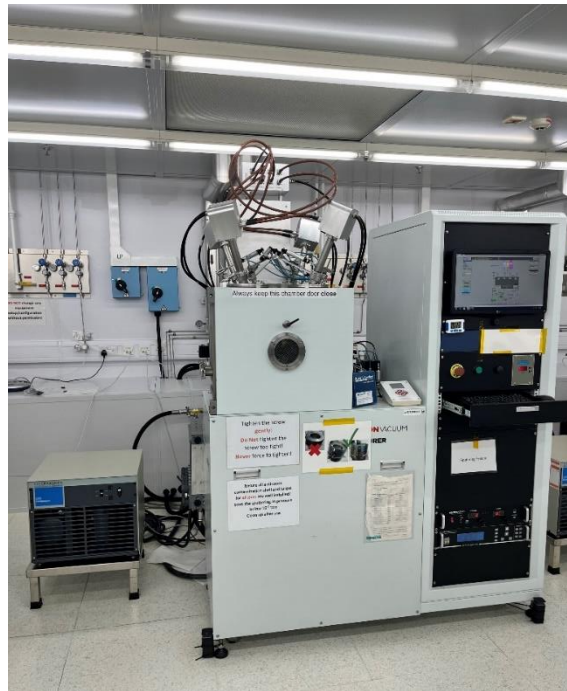
Figure 3.5 Sputtering machine used in the thin film coating.
