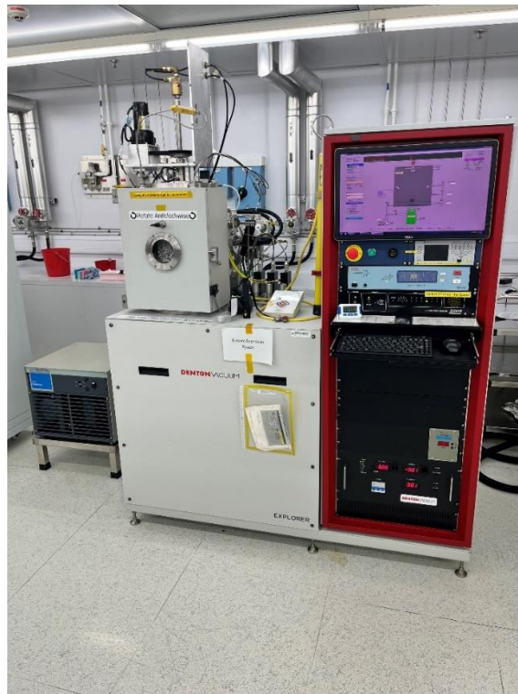
Figure 3.3 E-Beam Evaporation machine used in the thin film coating.
