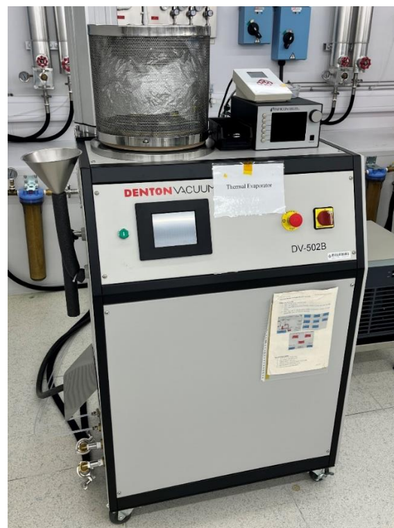
Figure 3.4 Thermal evaporation machine used in the thin film coating.
