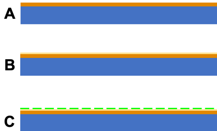
Figure 3.2 Schematic diagram of the fabrication process for the microchip for droplet generation, blue is glass, orange is metal thin film, yellow is insulating layer, green is SU-8 microstructure.
