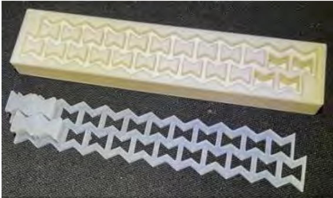
Figure 7.7: Trial of PLA mold and associated silicone band
