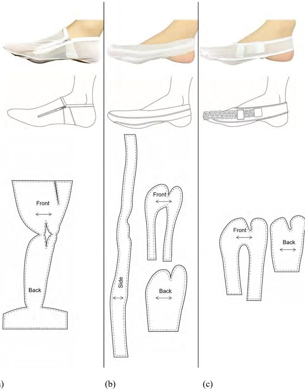
Figure 7.2: Design pattern and fabrication of the proposed sock-like orthosis (a) first prototype, (b) second prototype, and (c) final prototype
