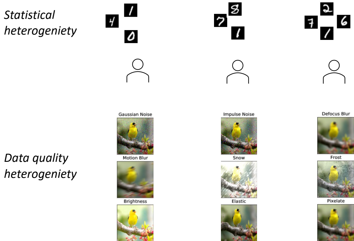
Figure 2.2: Data quality and statistical heterogeneity. The bottom of the figure shows the data quality heterogeneity on each client. Different corruption may appears on some of the data, thus, not all data are equal. The top shows the statistical heterogeneity on each client, where not all labels appears for a single client.
