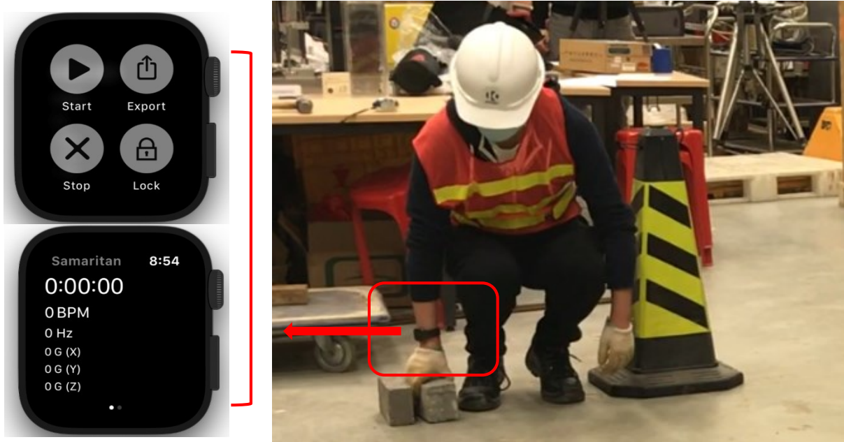
Figure 4-14 The Apple Watch placement ( right ) and data collection interface ( left )
