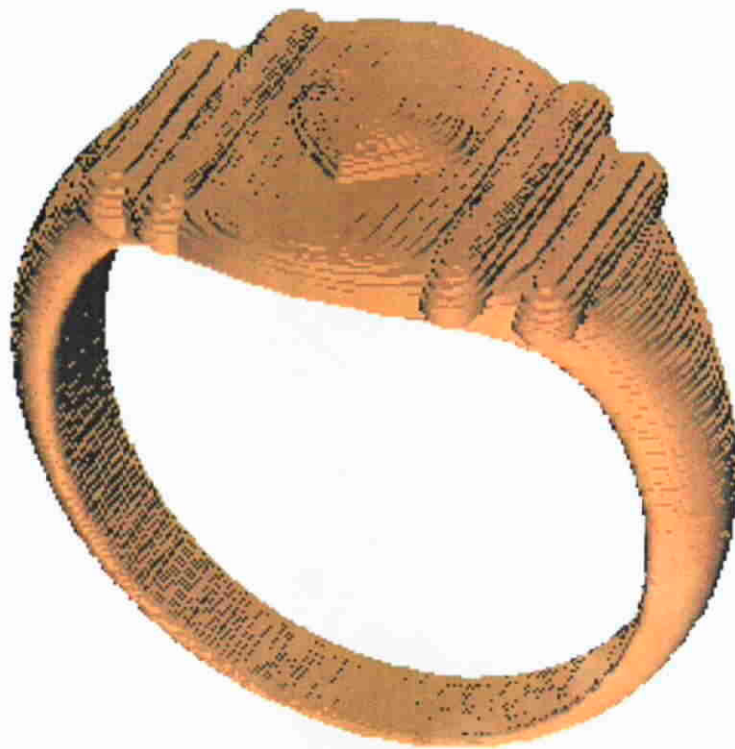
Figure 7-5. Vertical maximum inscribed slab model after bottom-up vertical slicing.
