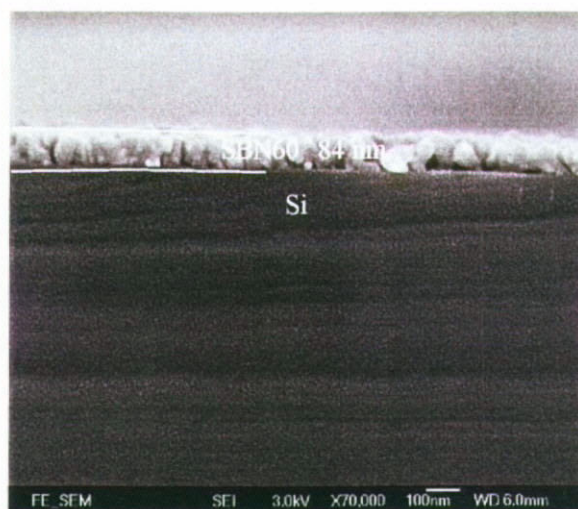
Fig. 6.2.3.1 SEM micrograph showing the cross-section of SBN60 film grown on Si substrate annealed at 700°C for 150 min.
