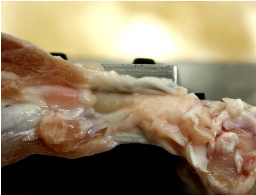
Figure 3-22. The sample was fixed by the fixation device with the AC surface facing the ultrasound transducer.
