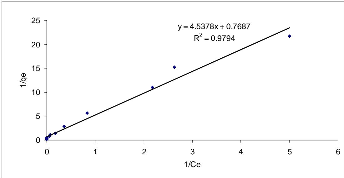
Fig. 4.3 Phosphorus adsorption data fitted to Langmuir equation
