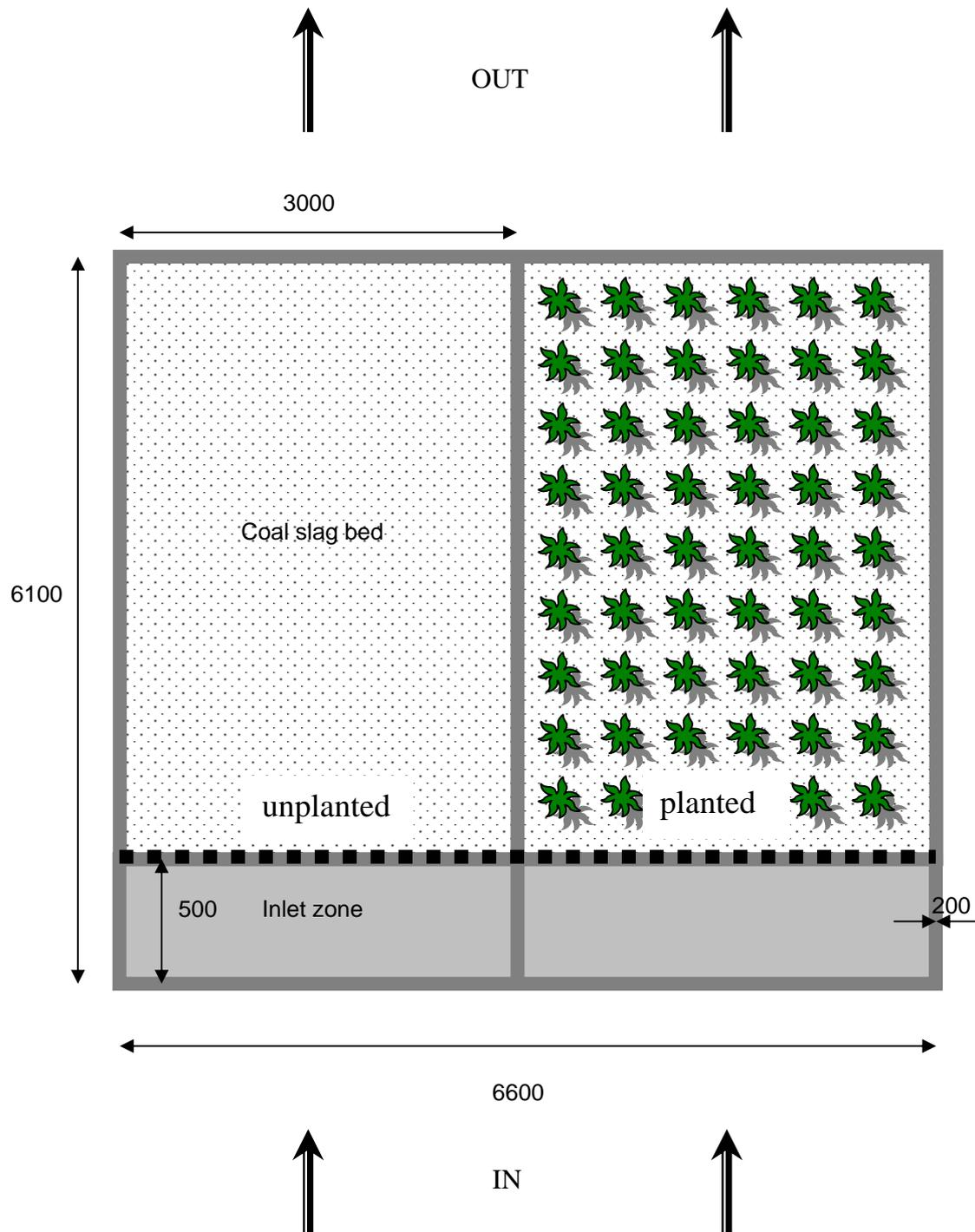
Fig. 3.3 Top view of the parallel pilot systems
