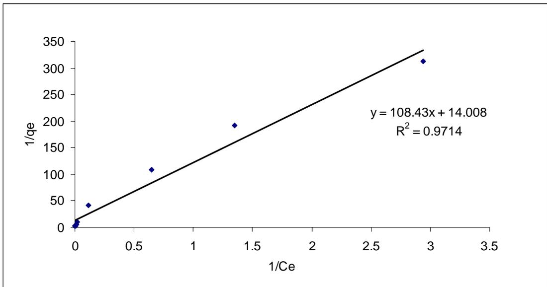
Fig. 4.4 Ammonia nitrogen adsorption data fitted to Langmuir equation
