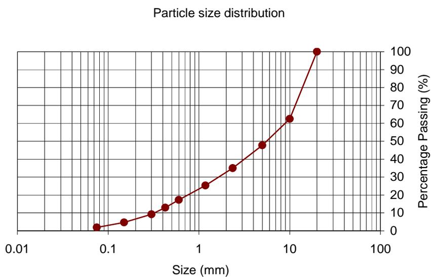
Fig. 4.1 Size distribution curve of coal slag
