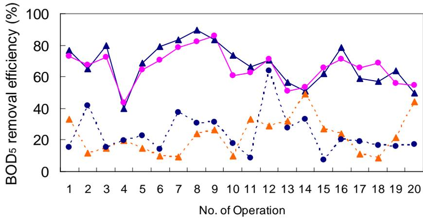
Fig. 4.6 BOD<sub>5</sub> removal efficiency in laboratory-scale system.
