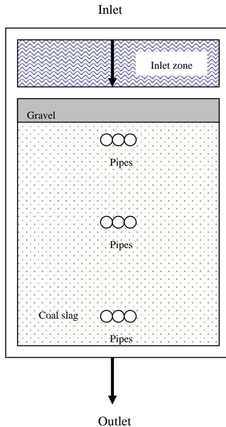
Fig. 3.9 Locations of pipes for D.O. measurement (Top view).
