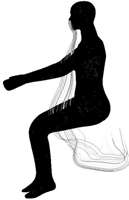
Figure 2.10 Path line showing origin of inhaled air in a stagnant ambient environment
