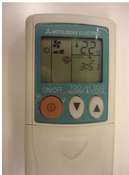
Fig. 4.6 The remote controller of a typical SRAC showing indoor air temperature setting
