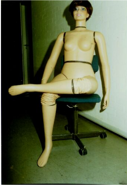
Fig. 5.4a Thermal manikin, height 168 cm (modeled after a typical Scandinavian woman)
