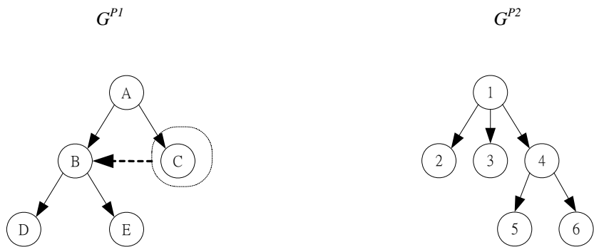
Figure 10(a): Start condition of GP crossover. Node 'C' of G^{P1} is mutated to connect to node 'E'
