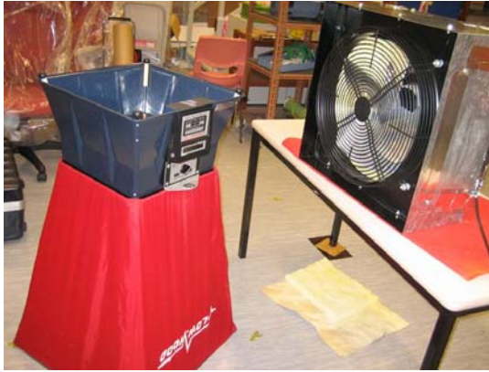
Figure 5.20: Measurement of volumetric flow rate of the propeller fan
