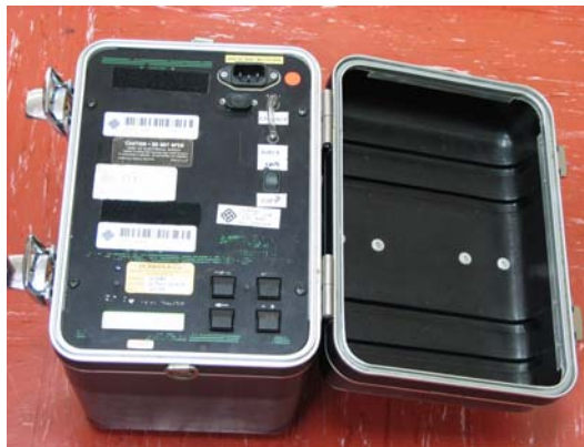
Figure 5.28: RAD-7 for radon measurement
