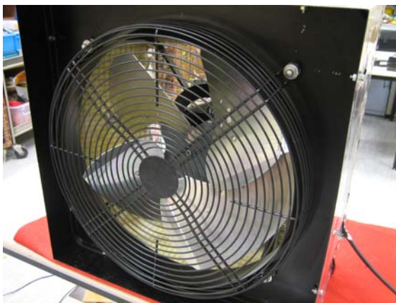
Figure 5.19: Propeller fan for make up air application
