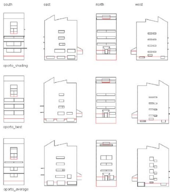
Figure 5.2: Alternative facade solutions generated by GS for one block of the School of Architecture in Oporto by Álvaro Siza. From (Caldas and Norford, 2001).
