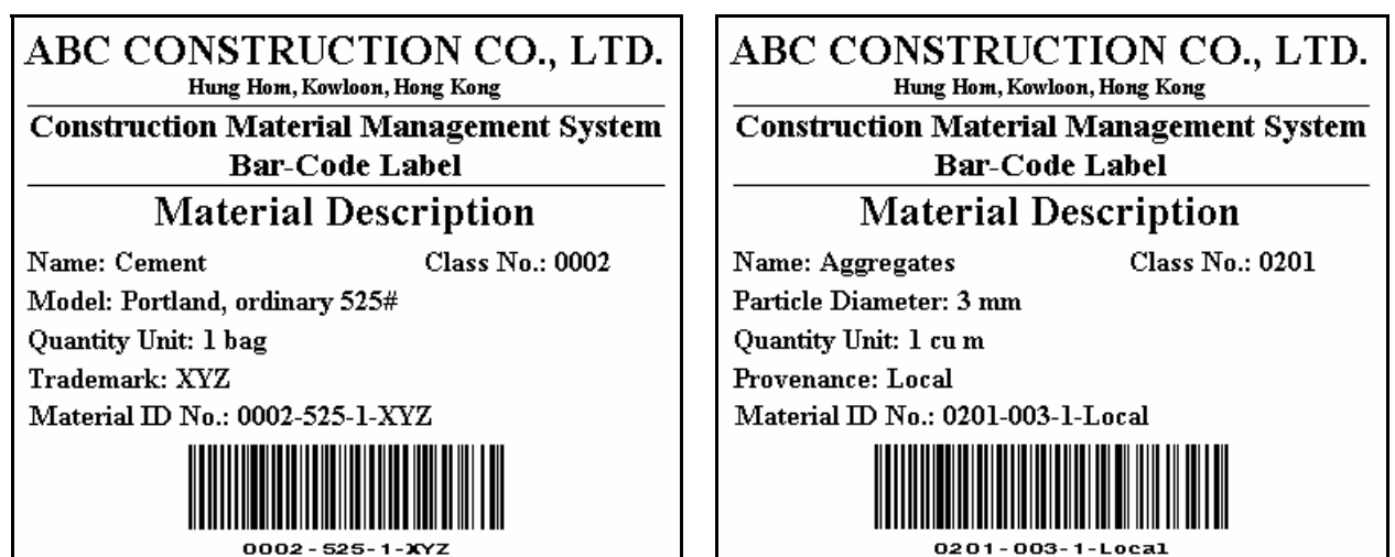
Figure 3.3: Sample bar-coding labels for construction materials
