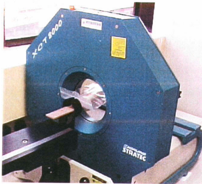
Fig 2.5b. Set up position for pQCT measurement of the fracture gap
