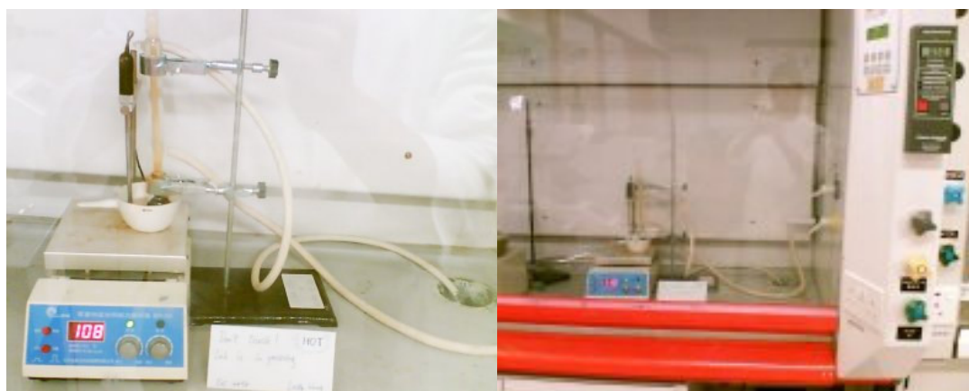
Fig. 9. Reflux setup inside fume cupboard
