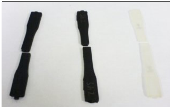
Fig. 27. Composite specimens after tensile test
