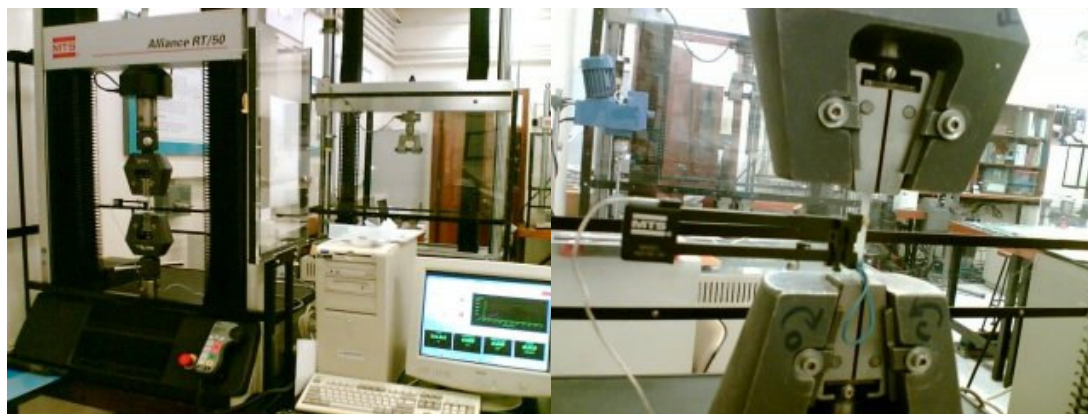
Fig. 13. 50kN MTS Alliance RT/50 tensile machine and extensometer
