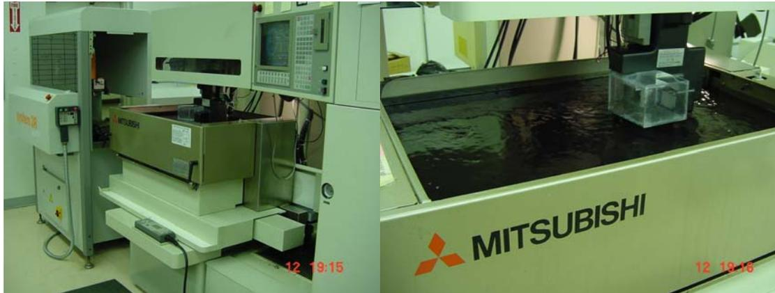
Fig. 2.2 A commercial wire electrical discharge machining (WEDM) equipment used to prepare our [112]-oriented Terfenol-D continuous fibers.
