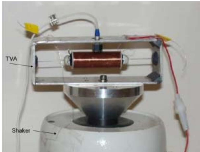
Fig. 5.6 Measurement setup for characterization of the smart TVA.
