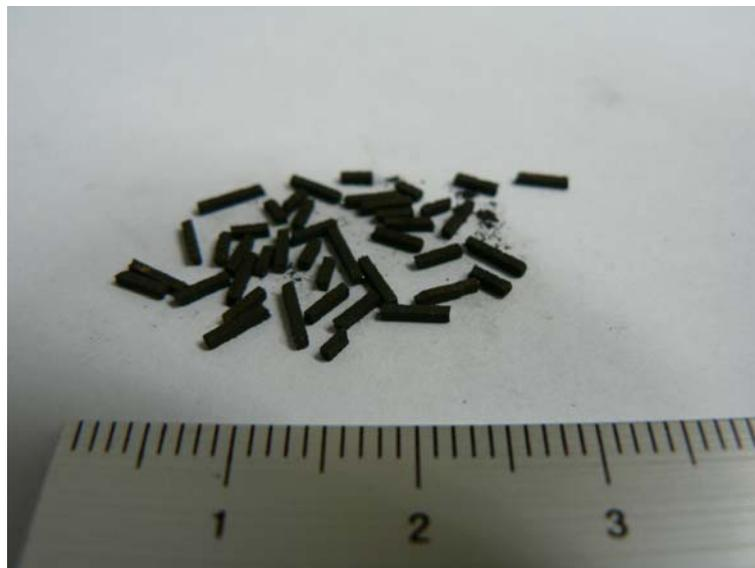
Fig. 2.6 Optical micrograph of [112]-oriented Terfenol-D short fibers for 4 mm long and (1 mm × 1 mm) cross-section.
