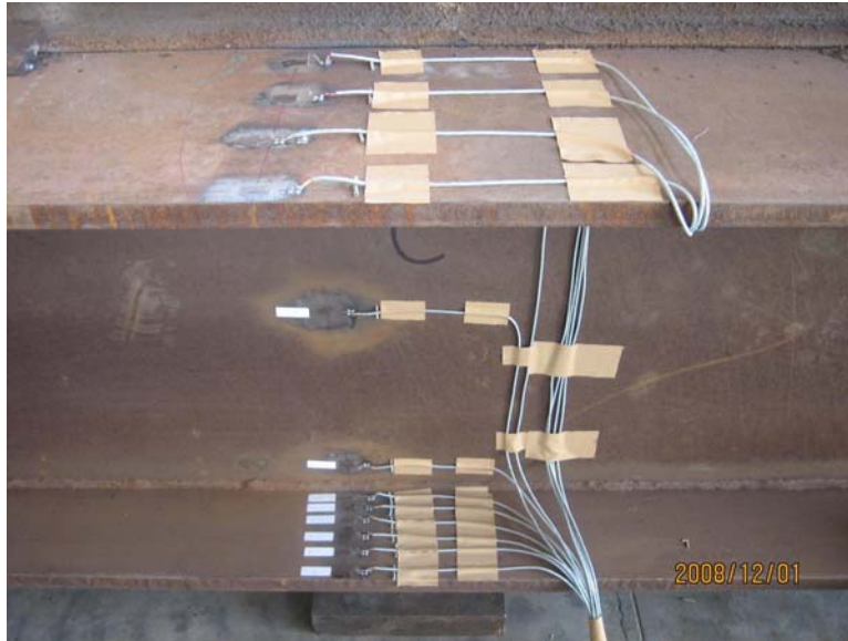
Figure 5.7 Photo of deployed strain gauges
