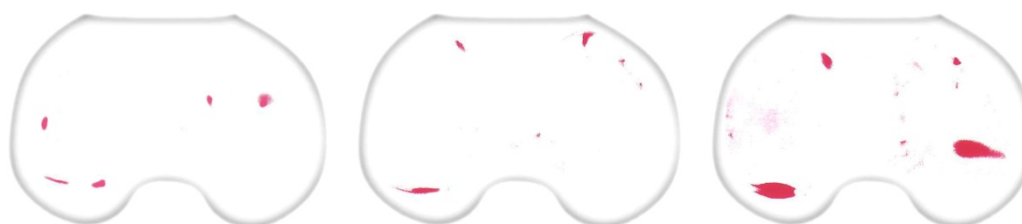
Fig. V-11 Pressure contour of Fuji film at 58.64N (left), 78.25N (center), 102.60N (right) compressive force.
