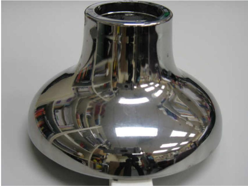
Fig. 6.11: The photo of 38% mineral filled PBT/PET blend after Sn/Co plating.
