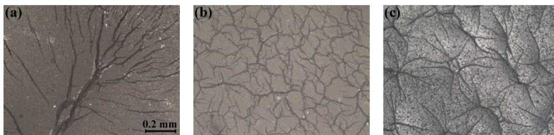
Fig. 5.8: Optical micrographs of swollen PC samples (dipping for 15 s) after etching in different NaOH concentrations and times (a) 2 M for 2 hr; (b) 4 M for 2 hr and (c) 6 M for 2 hr.
