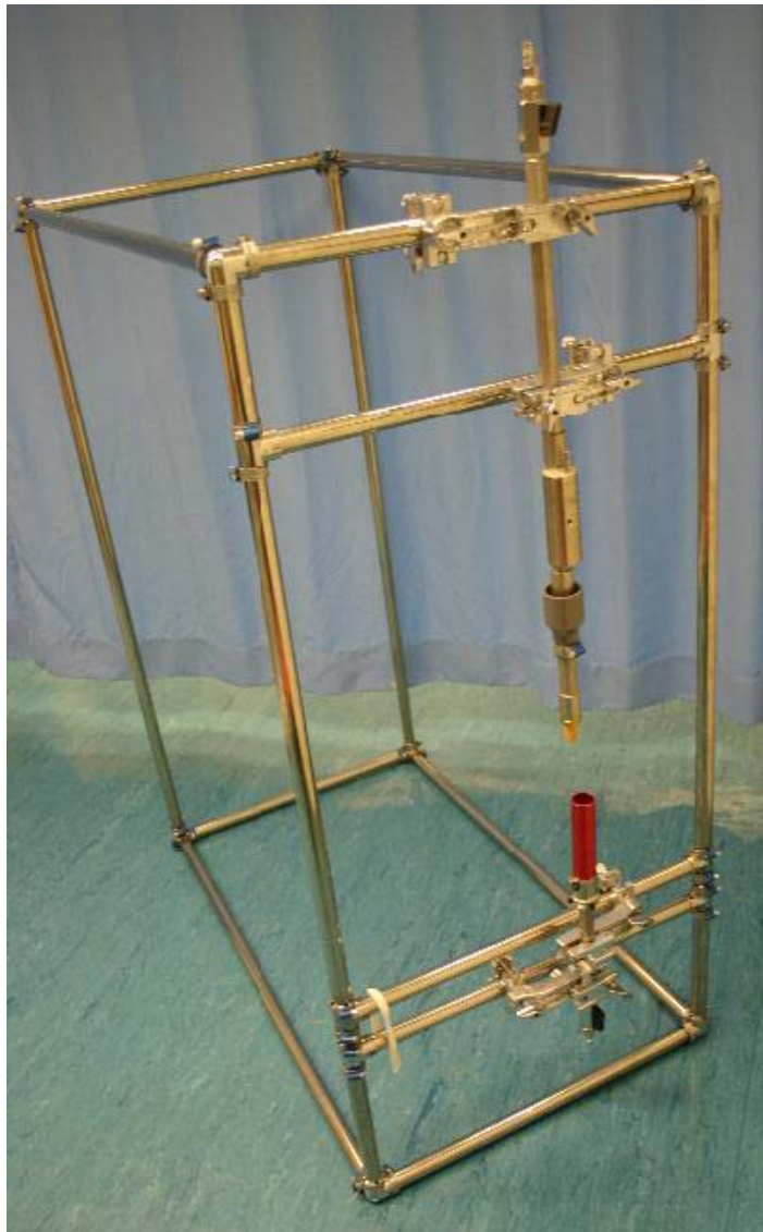
Figure A15. The alignment jig may be simply a rectangular metal frame comprised of common metal rods and joints. The structure can be dismantled and assemble for transportation. The casting and vacuum forming mandrels fix on alignment jig with metal clamp which is available in musical instrument store as a common connector for drum set.
