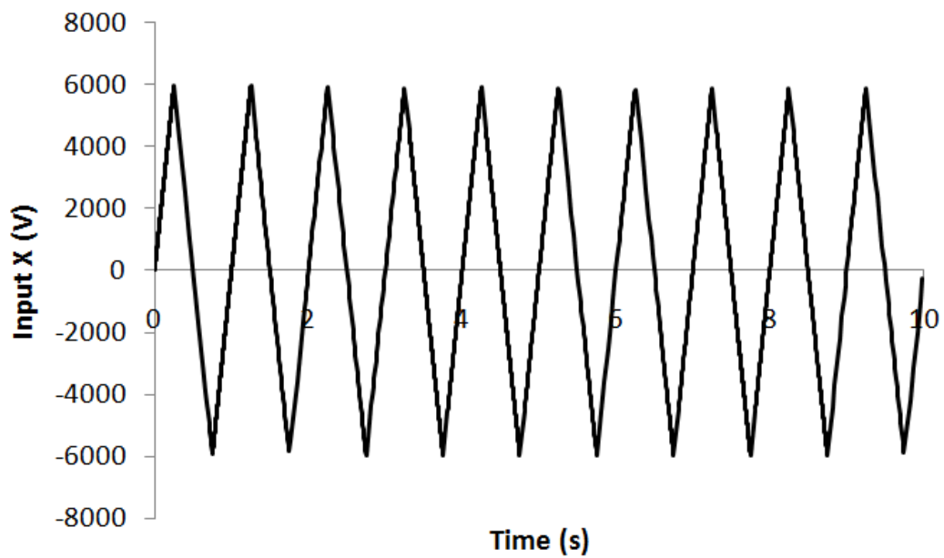
Figure 5-4. X Input of Closed Loop Nonlinear System with Electrode Dislocation using ASMC
