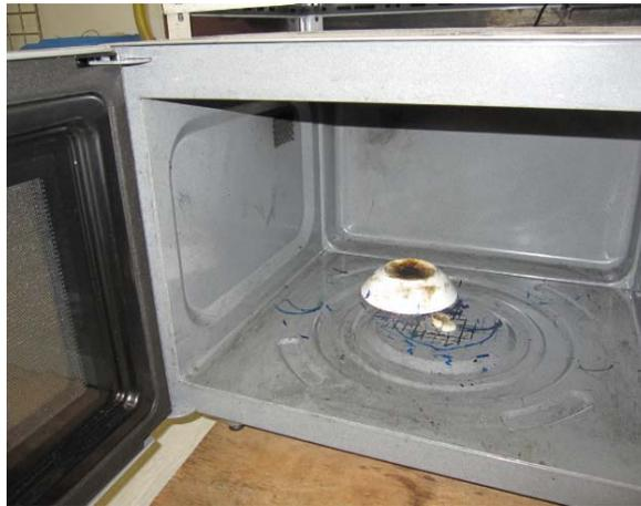
Fig.3.3 Image of the microwave oven for composite sintering used in this study
