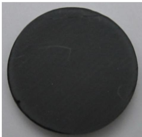
Fig.3.4 Image of the sintered (100:1:5 wt %) sample
