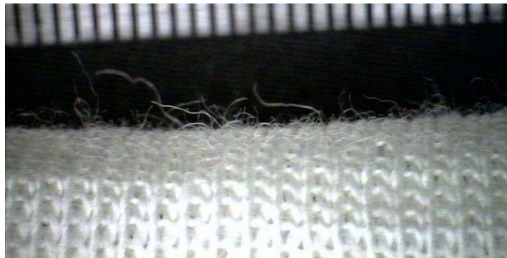
Figure.4.8 Fabric surface before brushing
