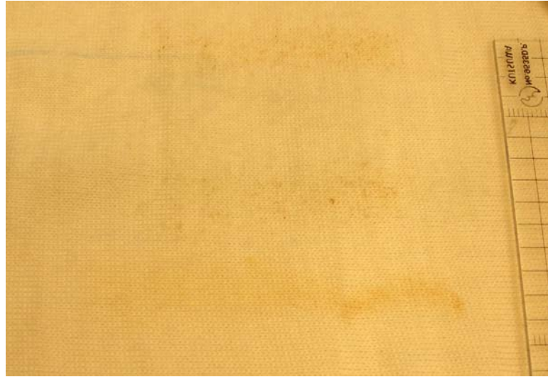
Figure 4.16 Wool fabric surface after pills cut by laser beam
