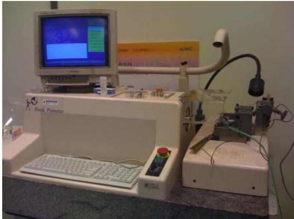
Fig. 3.12 SPDT machine (OptoForm 30, Advanced Optics Manufacturing Center, The Hong Kong Polytechnic University)
