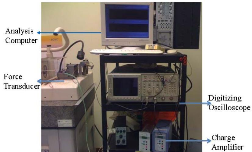
Fig. 3.19 Cutting force measurement system in single point diamond turning machine (Advanced Optics Manufacturing Center, The Hong Kong Polytechnic University)
