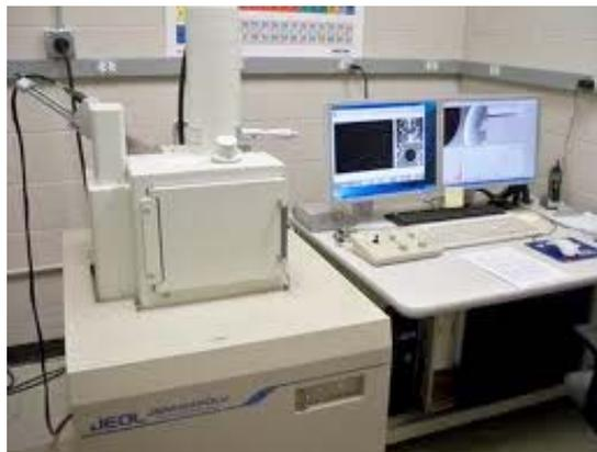
Fig. 3.7 Scanning electron microscopy (JSM-6490 JEOL)
