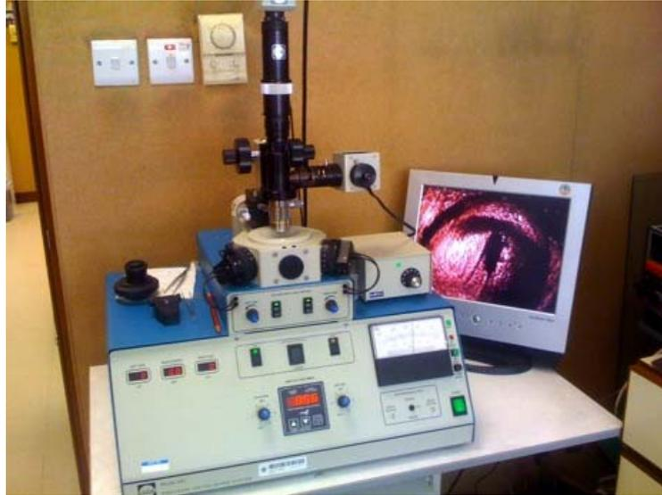
Fig. 3.10 Precision ion polishing system (Gatan 691)
