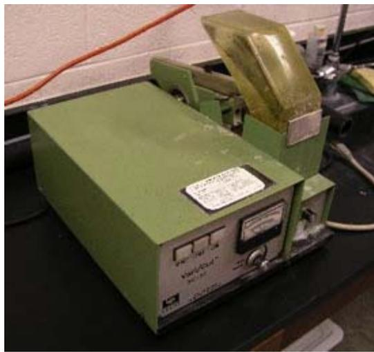
Fig. 5.1 Low speed saw
