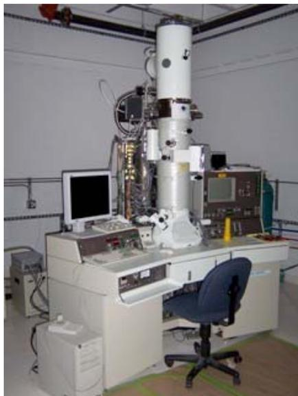
Fig. 3.9 Transmission electron microscopy (JEOL 2010F field emission)
