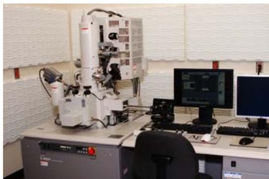
Fig. 3.8 Ultra-high resolution field emission scanning electron microscopy (Hitachi-S4800)
