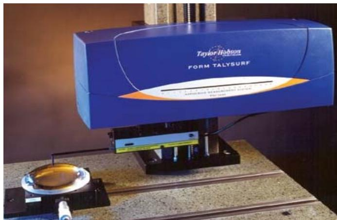
Fig. 3.16 Contact stylus type measurement system (Taylor Surf PGI 1240, Advanced Optics Manufacturing Center, The Hong Kong Polytechnic University)
