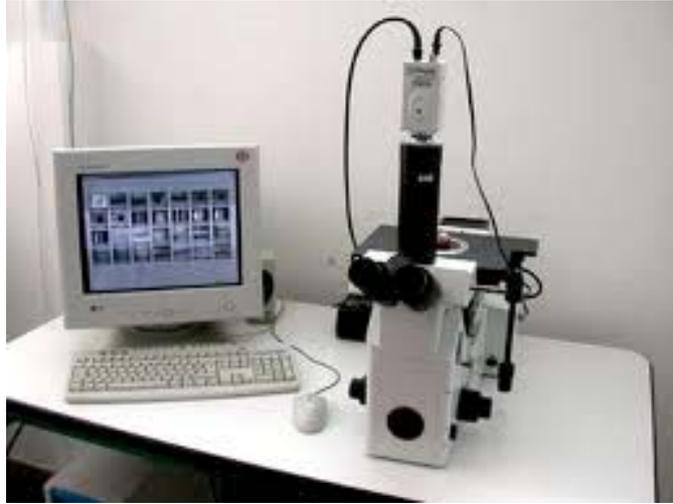
Fig. 3.11 Metallurgical Microscopy (Olympus GX 51, Shenzhen Tsinghua Graduate School)
