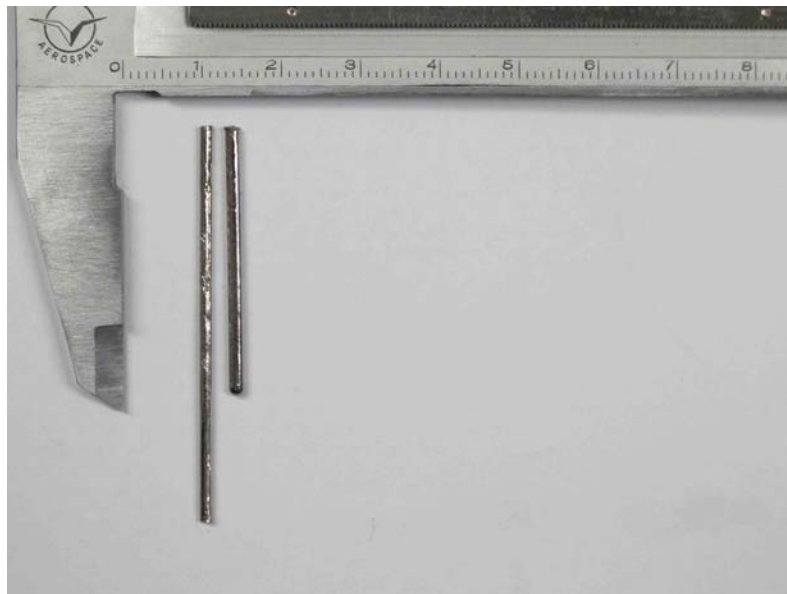
Fig. 4.1 Two sections of the as-cast Fe-based BMG (left) and Zr-based BMG (right) sample, respectively.
