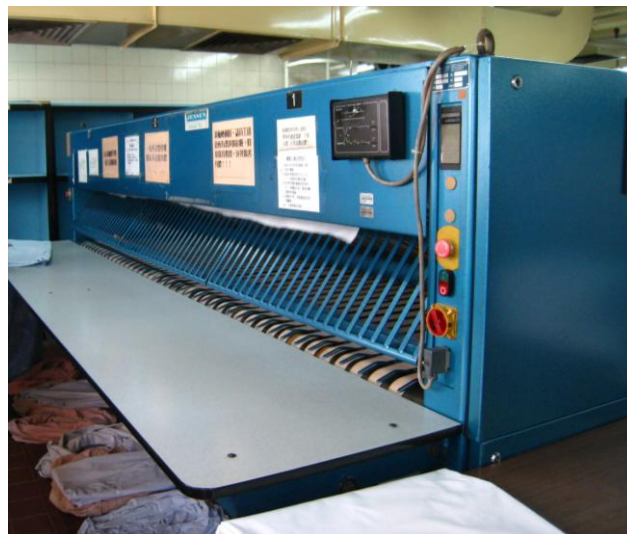
Figure 4.8 Flatwork ironer in the laundering section
