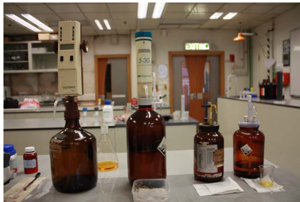
Figure 13 Equipment in testing COD
