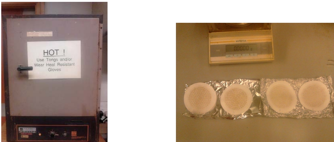
Figure 14 Heating machine and filter paper for testing MLSS
