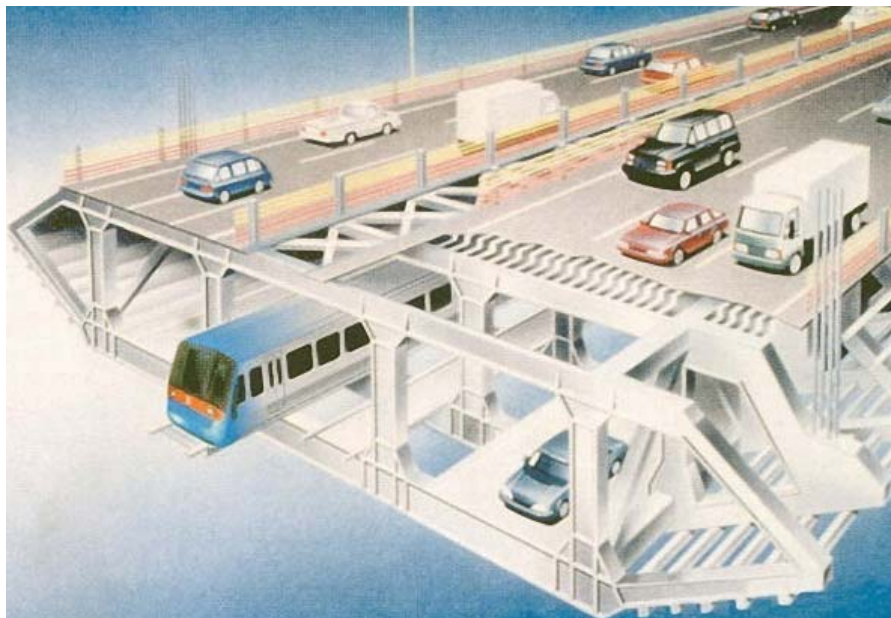
Figure 5.6 Schematic configuration of Tsing Ma Bridge decking system (Wong, K.Y. 2007)
