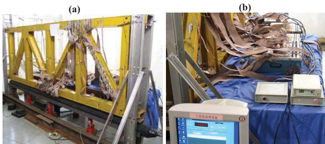
Figure 4.2 Overview of laboratory test set-up: (a) steel truss specimen (b) test instruments
