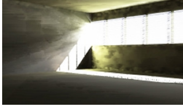
Figure 4.8. A Radiance rendering of the classroom under clear sky, tilt angle = -30^\circ , solar altitude = 60^\circ , solar azimuth = 50^\circ west of south.
