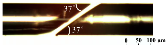
Fig. 5.13 Photo of the aligned angled fibers in characterizing the ROTE sensor.
