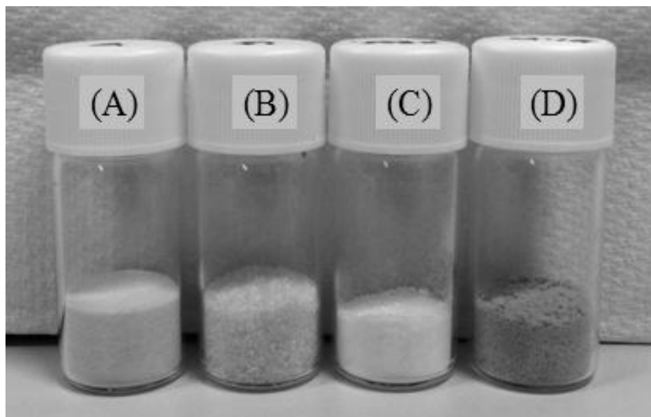
Figure 6.3 Images of (A) agar powder; (B) gelatin powder; (C) gallic acid; and (D) gallic acid loaded agar/gelatin microcapsules
