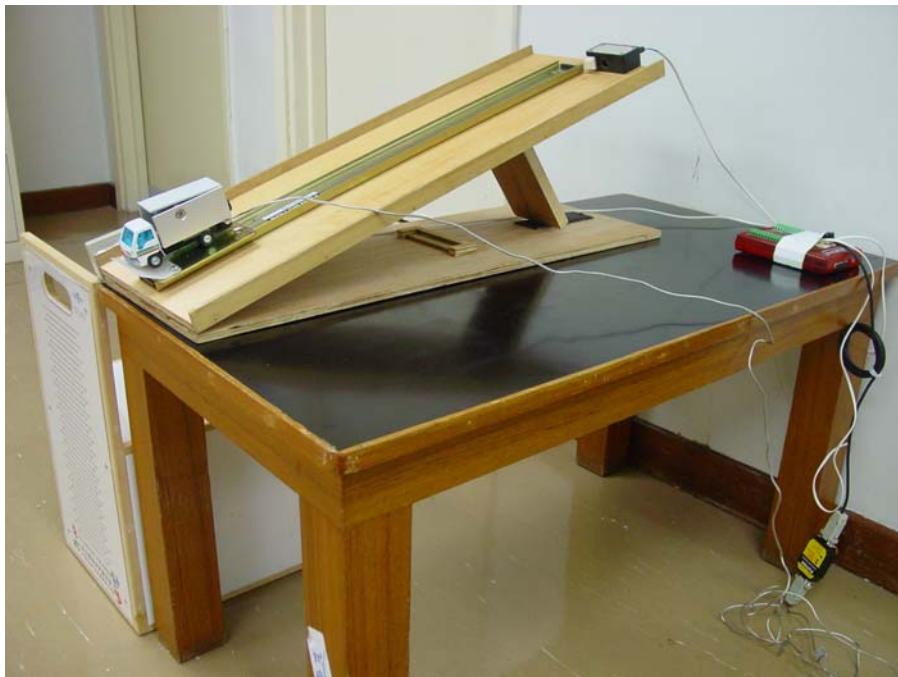
Figure 3.6 b. The programmable input-output controller was attached to the 2 buttons on the slanted board and the load cell in the trunk of the toy car.
