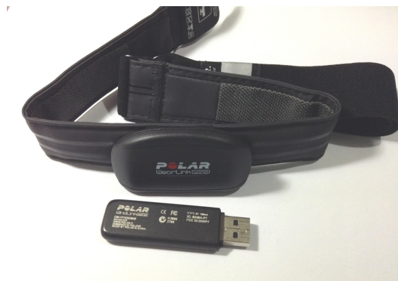
Figure 4.2. Picture of heart rate monitor, chest belt and infra-red receiver.
