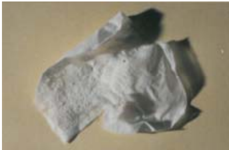
Figure 4.29 Different textures of polymers extracted from activated sludge.
