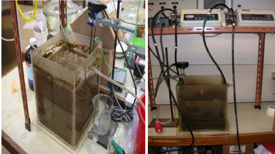
Figure 3.3 Biological reactors of 10 liters effective volume.
