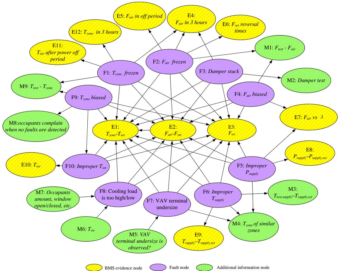
Figure 9.2 Diagnostic Bayesian network for fault detection and diagnosis of VAV terminals
