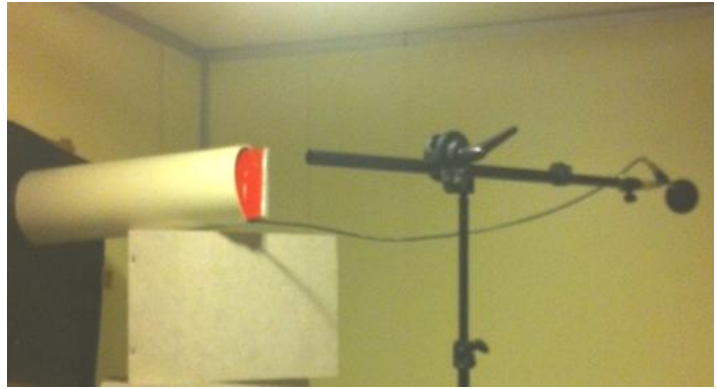
Figure 6- 6 Acoustics tests (with absorber in the ventilated duct) when the microphone put in the room.
