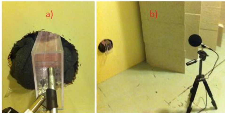
Figure 5- 6 Noise measurements a) in the duct and; b) noise measurement in the room.
