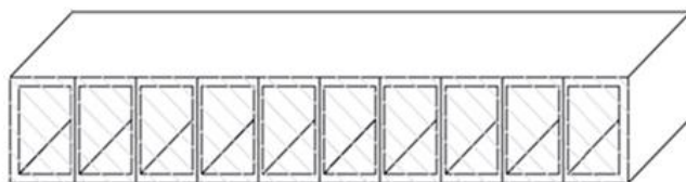
Figure 1- 3 Multiple quarter-wave resonators.
