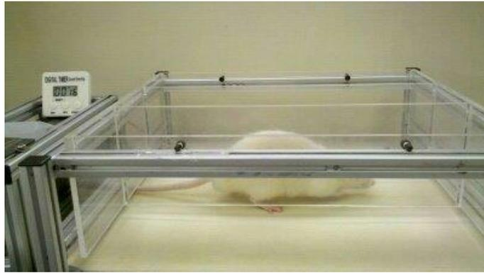
Figure 3.3 Treadmill (KN-73, Natsume Ltd., Japan) used in the study with a speed adjustment from 0 to 30 m/min.
