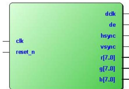
Figure 35 Structure of HDMI timing module.
